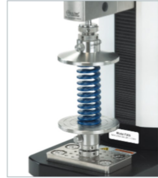
Compression spring testing
