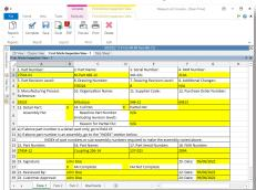
First article inspection view in Real-Time or Process Analyzer provides a clear and concise approach for completing FAI reports that align with the AS9102 requirements. This feature includes forms 1, 2, and 3 with options to export to Excel or PDF and allows users to search first article inspection information and production data in one location.
